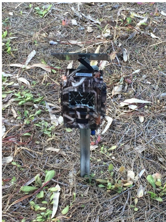
Figure 1. Reconyx PC900 camera trap mounted on peg
