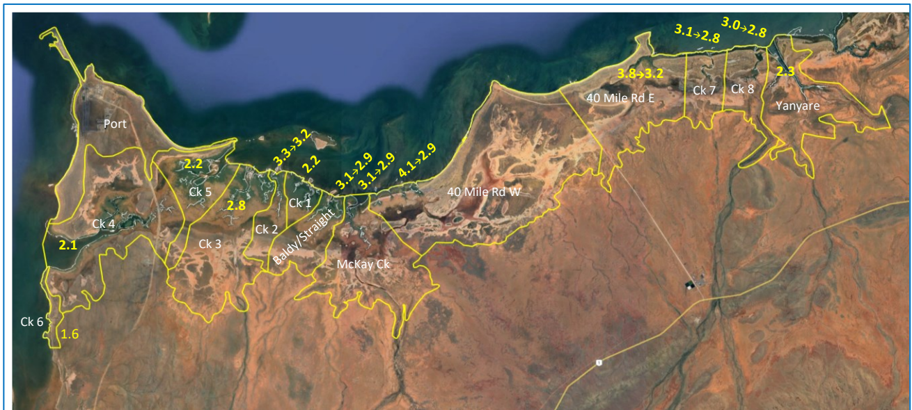
Figure 26. Calculated Vs:Vc ratios for the natural catchments. For those catchments where the ponds of scenario 7.2.1, the first number is the natural ratio, and the number after the arrows is the new ratio with the ponds (Larcombe, 2024).
