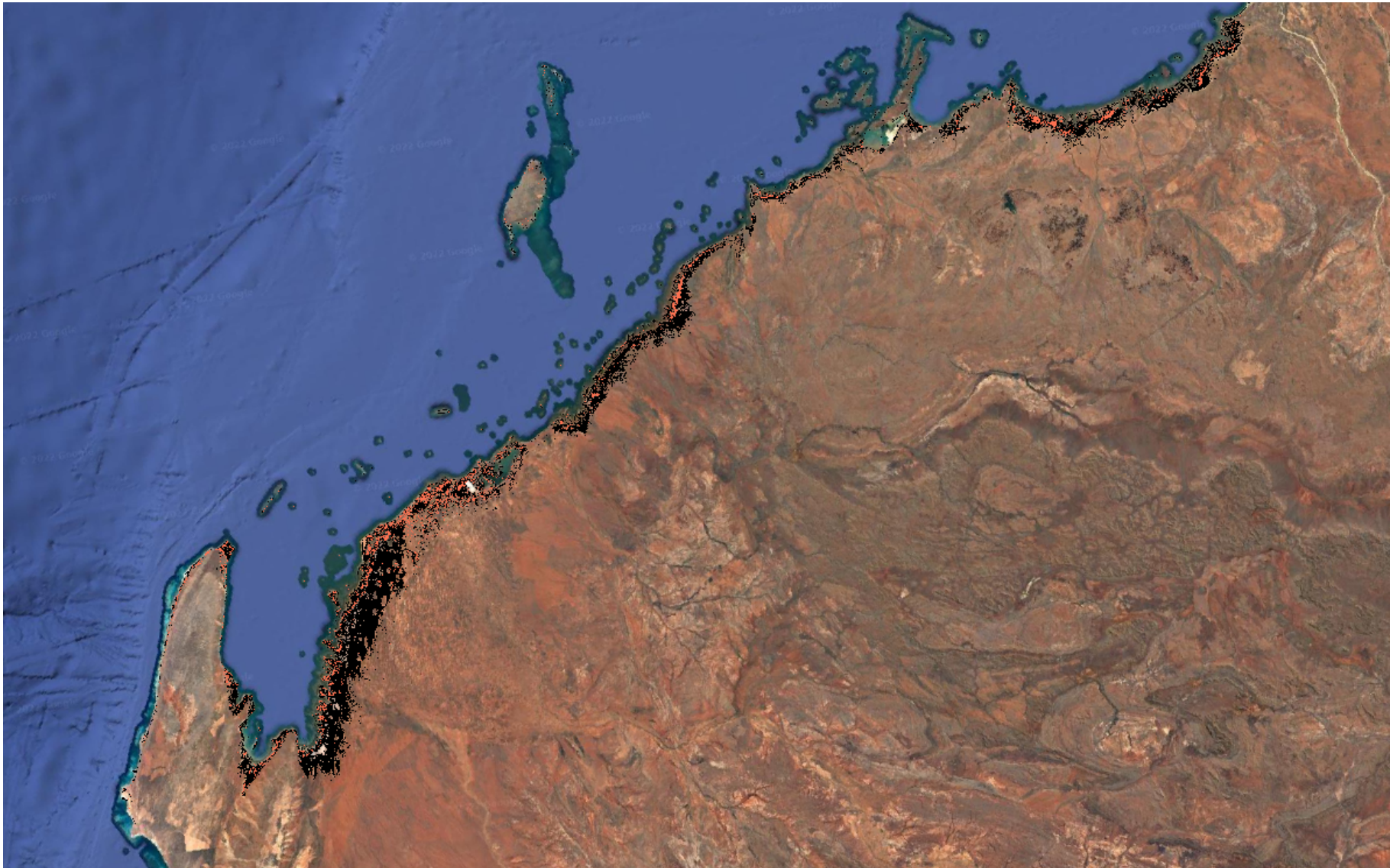
Figure 9. 2021 SVM derived algal mat (black) and productive algal mat (orange) based on MAX NDVI \geq 0.4 and STD NDVI \geq 0.04 .
