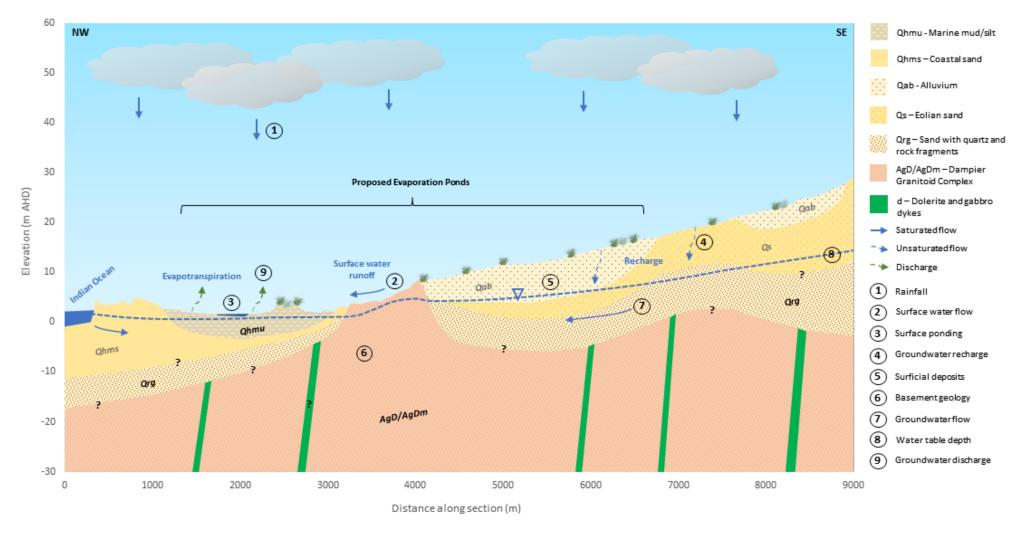
Figure 4-33: Conceptual hydrogeological model
