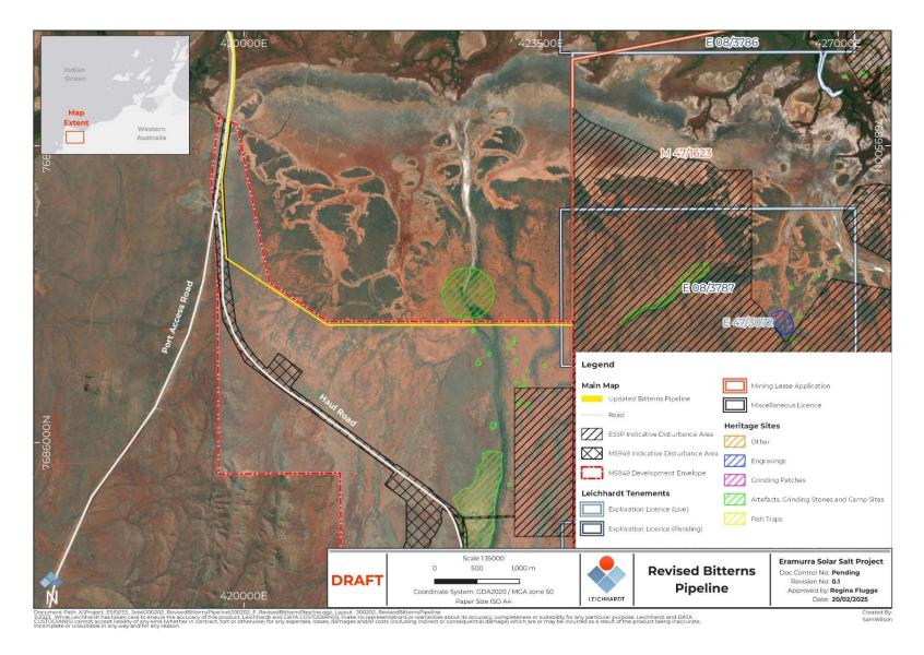
Figure 1-4: Bitterns discharge pipeline route and port haul road
