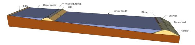
Figure 1-8: Typical embankment sections
