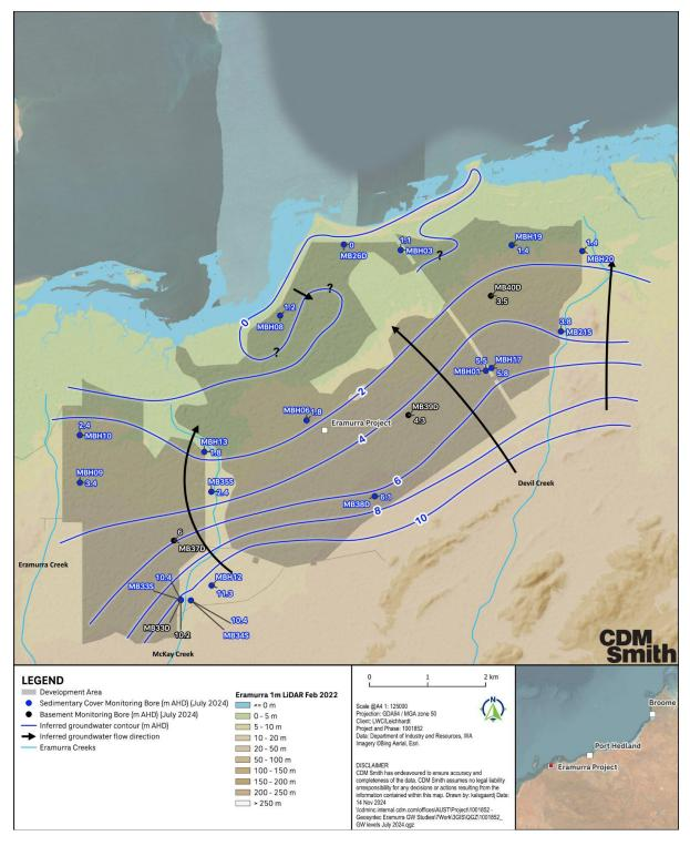
Figure 4-34: Inferred groundwater elevation contours and flow direction (July 2024)
