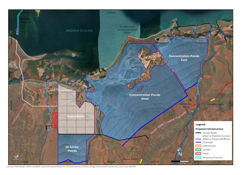
Figure 1-7: Pond layout and configuration
